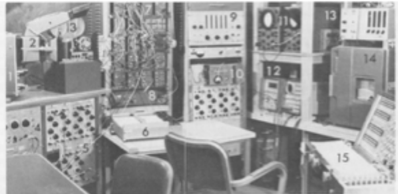
FIG. 1-21. A modern EEG and perceptual laboratory, equipped for EEG, average evoked potential, and CNV recording. 1. Tektronix 502 oscilloscope; 2. Tektronix Polaroid camera; 3. Grass Kymograph camera; 4. Grass physiological stimulators; 5. Tektronix power supply, waveform and pulse generators; 6. Moseley X-Y plotter; 7. Massey-Dickinson control and programming equipment; 8. Power supply; 9. Hewlett-Packard counter; 10. Taperreader; 11. Oscilloscope monitors; 12. Mnemotron computer of average transient (CAT) and accessories; 13. Preset controller and tape coder; 14. Ampex FR-1300 7-channel FM tape recorder; 15. Grass Model 6 8-channel EEG.
